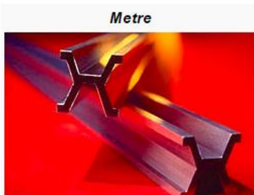
Historical International Prototype Metre bar, made of an alloy of platinum and iridium, that was the standard from 1889 to 1960.
